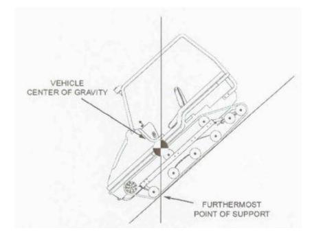
When the vehicle's center of gravity passes this point, the vehicles will tip over SUDDENLY.
