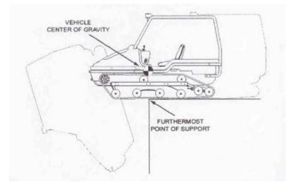
A tracked vehicle can climb or descend slopes so steep that the vehicle can tip over, forward OR backward before it loses traction. Tip-over occurs when the vehicle's center of gravity passes across an imaginary line drawn straight up from the furthermost point of support with the ground.
