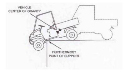
A tracked vehicle, however, will continue on without any warning until its center of gravity passes across an imaginary line drawn straight up from the furthermost point of support with the ground. It will then drop SUDDENLY. (See illustration). THIS WILL HAPPEN EVEN AT THE VERY SLOWEST OF SPEEDS.
